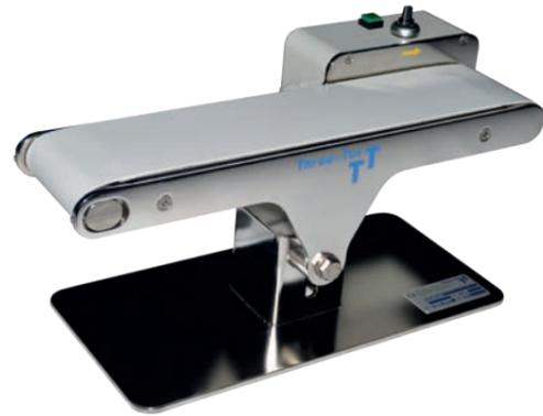
The conveyor belt is suitable for gentle removal and cooling of the extrudate. In order to achieve more efficient cooling of the extrudate, a cooling tank can optionally be integrated on which the belt rests and is continuously cooled. This enables the haul-off of extrudates with a temperature of up to 300 °C. The belt speed can be variably adjusted between 0 and 15 m/min.
