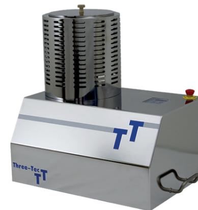
The Spheronizer is used for reducing the length and rounding off fine extrudate strands. The desired geometry of the end product is influenced by the batch size, the speed and the surface structure of the friction disc. Depending on the container size, a batch quantity of 5 to 5,000 grams can be processed.
