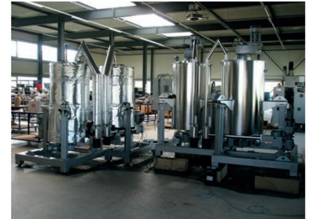
Battery production feeding systems completely insulated
