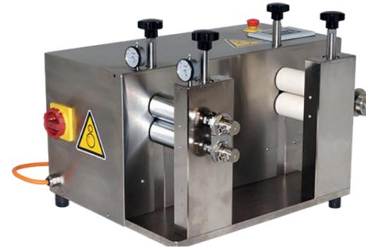
The film roller from Three-Tec enables the calibration of flat, dry extrudates. Furthermore, round extrudates can also be rolled into a film with a defined thickness. Subsequently, the product is evenly wound onto a spool. The film roll consists of an adjustable and temperature-controlled pair of rolls, an adjustable pair of tension rolls and a rewinder, or spool.
