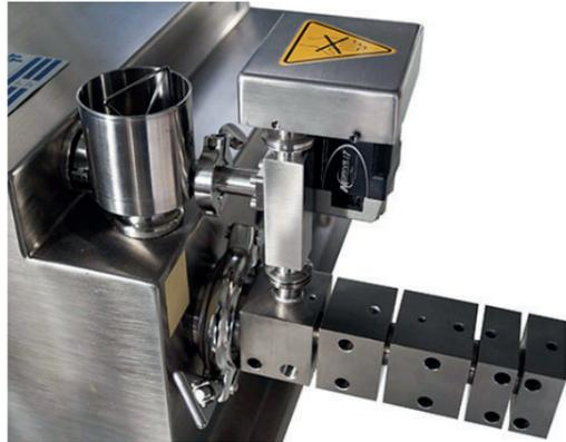
Stuffing feeding devices are used for the reliable feeding of very poorly feedable or very cohesive and very light products into an extruder. With the stuffing feeding device, products are pressed into the barrel of the extruder from above.
