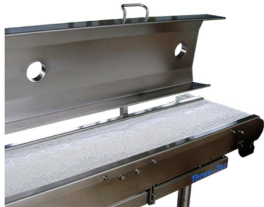
The cooling conveyor belt is suitable for the gentle removal and efficient cooling of extrudates and granules. The conveyor belt rests on actively cooled cooling elements and is permanently cooled during operation. Air connections in the lid of the cooling conveyor belt allows additional air cooling of the product. The belt speed can be variably adjusted between 0 and 20 m/min.
