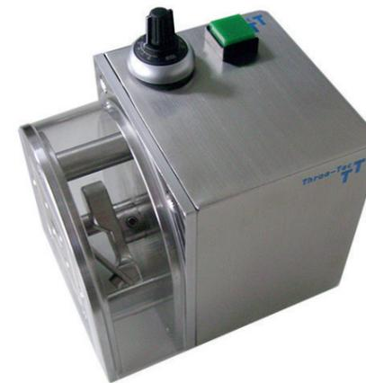
With the hot cutter, the extrudate can be reliably processed into pellets or granules with one or more knives in direct contact with the die plate. Both wet and melt extrudates can be processed. The number of knives used and the speed setting allow the production of pellet lengths or pellet sizes between 0.5 and 10 mm.
