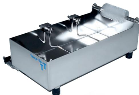
The cooling bath in different lengths and designs is used for efficient cooling of various extrudates before further processing by means of a winder or pelletizer. It is equipped with holding-down bars or holding-down rollers and scraper brush and mounted on damping elements. The water can be drained via a valve. In our larger cooling baths, a cooling unit can be connected and the water level is adjustable.
