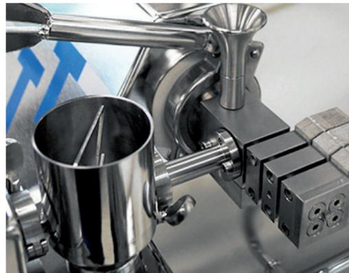
Side feeding devices are used for the forced feeding of powders and granules into an extruder. Three-Tec manufactures side feeding devices for all extruder sizes and throughput ranges.
