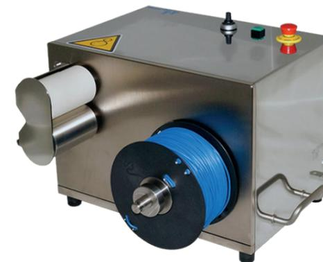
The filament winder from Three-Tec is suitable for winding the extrudate onto a spool. The tensile force between the take-off roller and the spool is adjustable, which enables very uniform winding. In addition to round strands, the winder can also be used to wind ribbon-shaped extrudates onto a spool. The filament winder is controlled by means of an integrated potentiometer.
