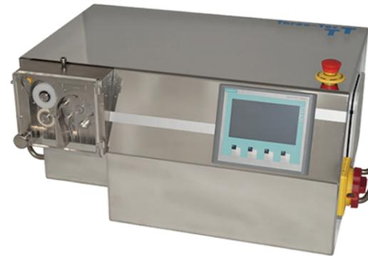
The pelletizer can be used to process strands into pellets or granules. The speed of the feed roller and the cutter are independently adjustable. This allows the extrudate feed to be perfectly matched to the extrudate and the pellet length or pellet size to be adjusted between 0.5 and 10 mm during processing.
